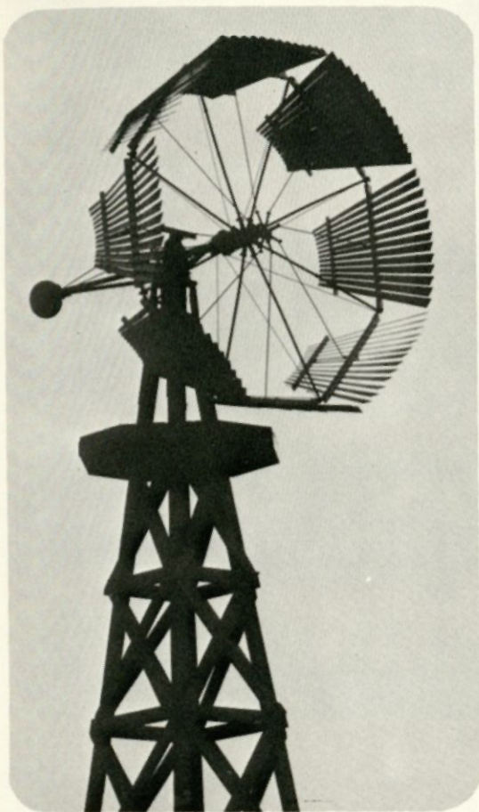
The Duplex power windmill breaks the skyline. 14½ foot diameter wheel and rated by manufacturer at 12 h.p. used . . .
