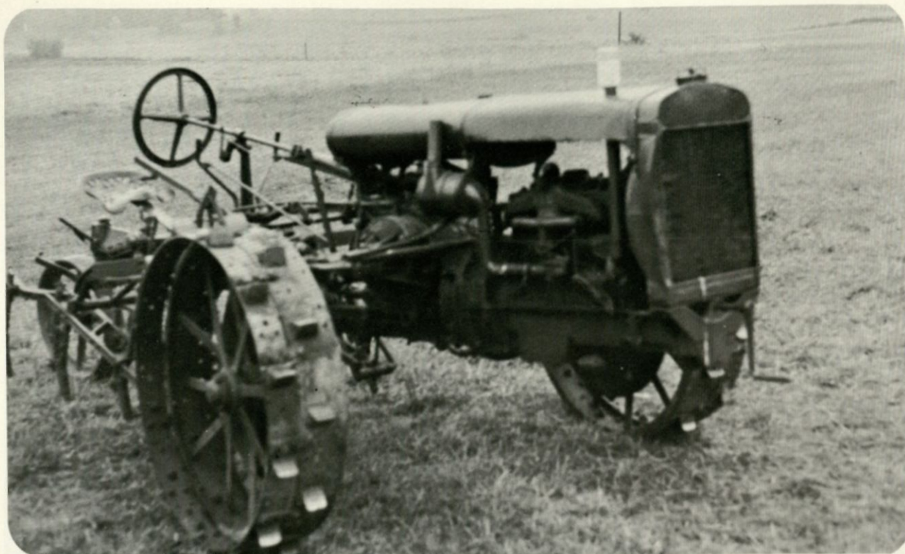
A Rumely DO-ALL. This was one of the first attempts to produce a row crop tractor.
