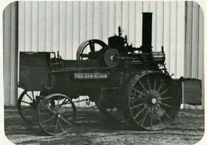
30 h.p. New Huber. All steam engines made by the Huber Co. were called "New Hubers".
