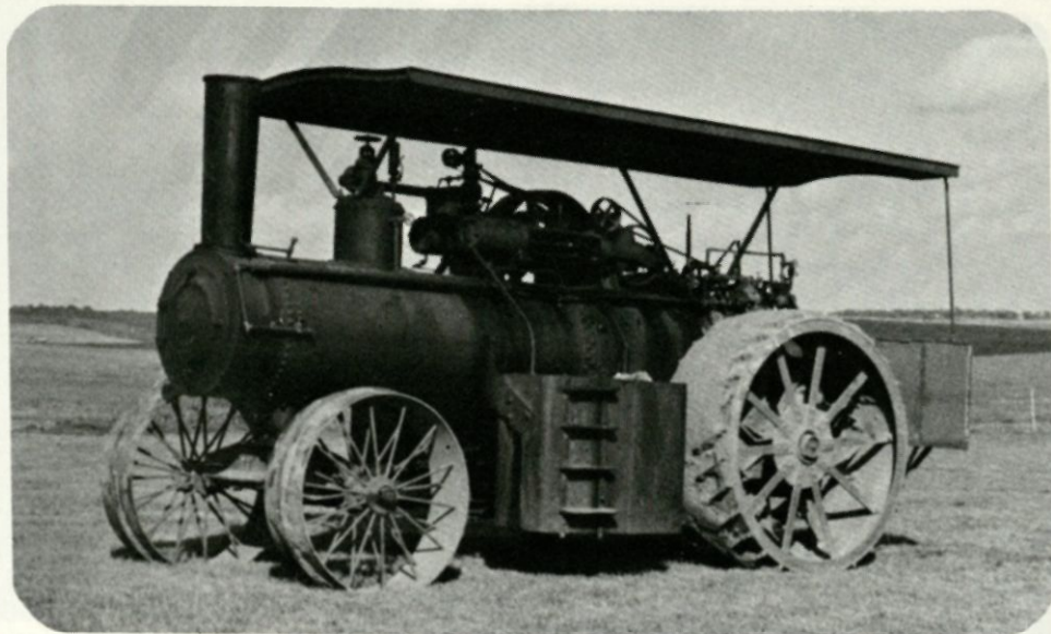
Curtis Leighty of Rochester, Mn. owns the 30 h.p. Double Rumely. Used for threshing during its working days.
