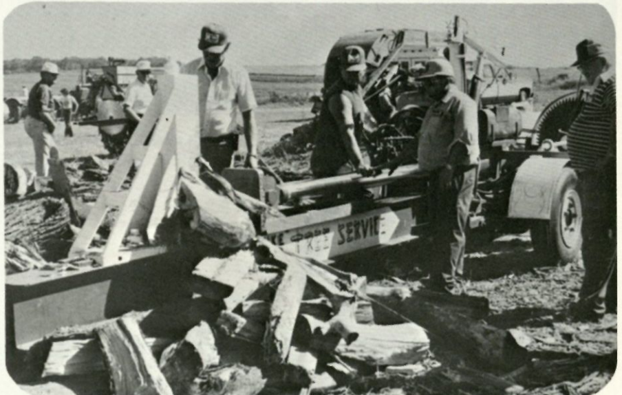
DeWayne Michaelson of Morris, Mn. built this log splitter from scratch. It has 8 inch cylinder, 9 inch travel and pushes 33 Ton. It will split a 50"x90" log.
