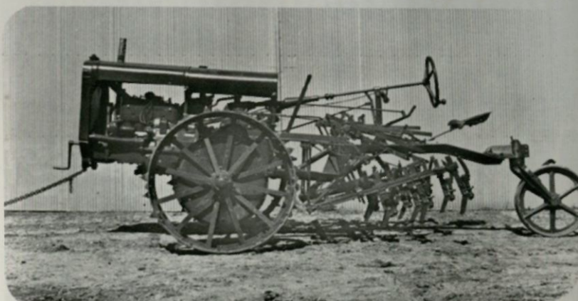
Rumely DO-ALL. An early attempt at a row crop tractor. Dale Akerman of Ashby owns this unique tractor.
