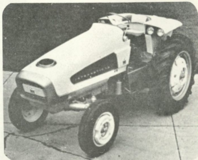
1961 HT-340 Experimental Tractor featuring gas turbine and hydrostatic transmission.
