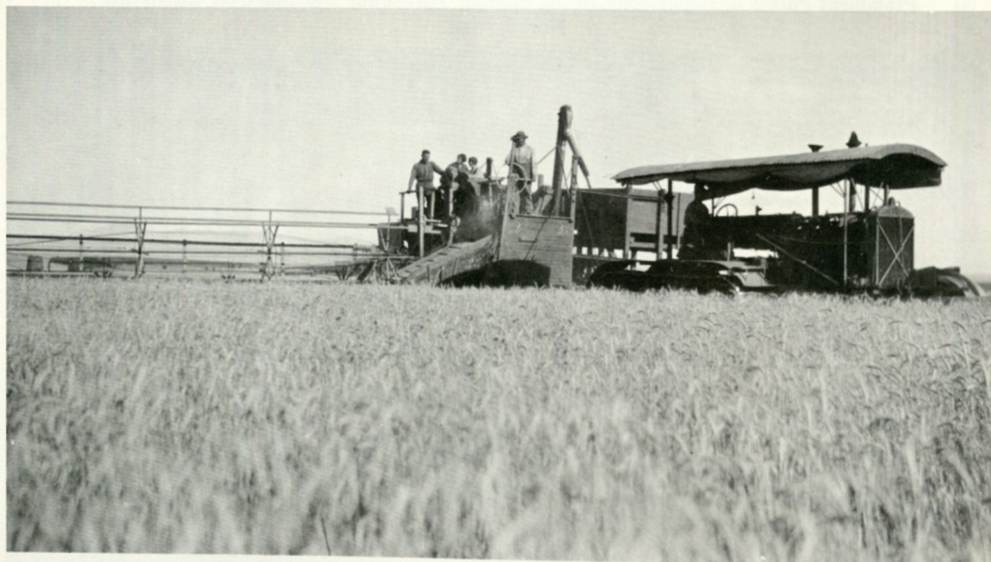
75 h.p. Best pulling a ground power 24 ft. harvester near Great Falls, Montana in 1922.
