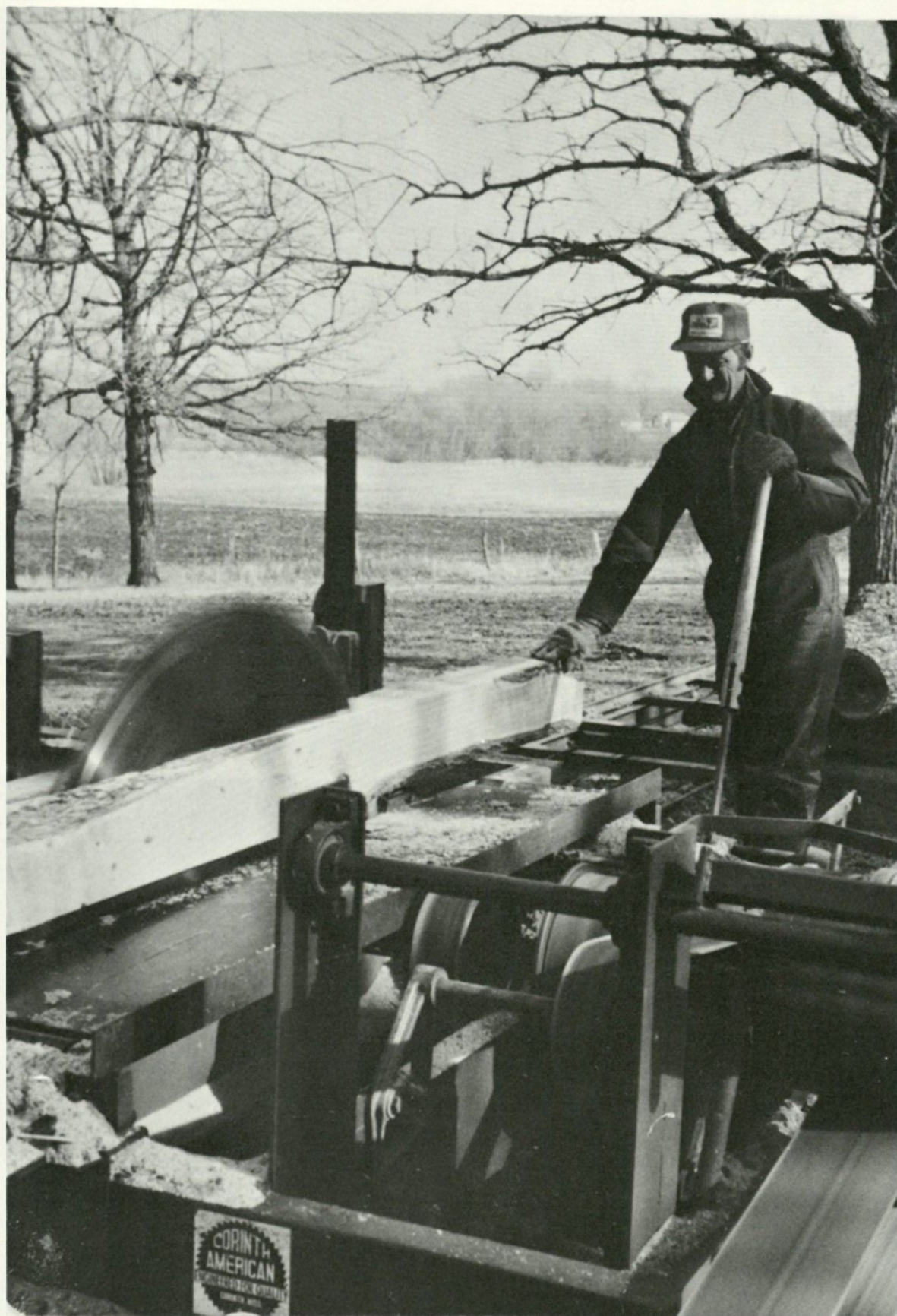
Ken Aasness sawing in Dane Prairie Township about 1980. This is a right-hand mill, belt powered. Most of the smaller mills are left-hand mills, powered by power takeoff from a farm tractor. Dane Prairie had a number of sawmills in the early 1900's. The Skinrud Brothers ran a mill powered by a Northwest Steam Engine. Henry Skinrud was a member of the Lake Region Pioneer Threshermen's Association. Also Jens Jensen and Alex Olson operated their own sawmills.
