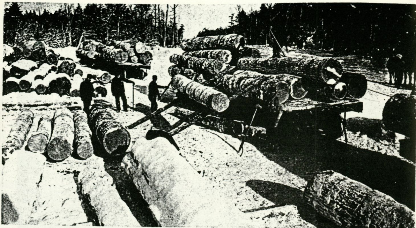
Cross haul loading was common in the early days. Horses furnished power to the cable which can be seen around the log half-way up on the skids. The man with cant hook was called a "sender-upper". He had to be skilled to make sure the log was "cut" at the right moment to land properly on the load. This was necessary where one end was bigger and thus traveled faster.
