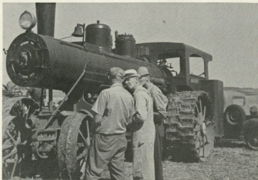
Henry Johnson's 22 H.P. Avery undermounted steam engine. The engine was mounted on a frame under the boiler. This took the strain off the boiler, similar to the locomotive on the railway.
