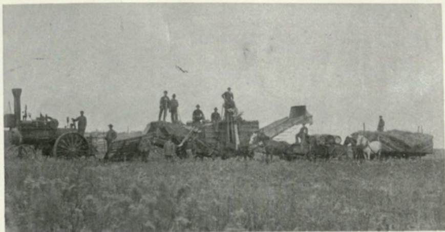
Picture of small Advance steam engine and hand feed and straw carrier separator taken near Kensington, Minn. around the turn of the century. Notice the staw cart behind the engine and the water wagon with barrels on top. They were filled from the tank and gave a supply of water while another load of water was pumped from a lake or slough. Note the straw wagon filled with straw. This was used to fill the cart behind the engine when moving from place to place.
