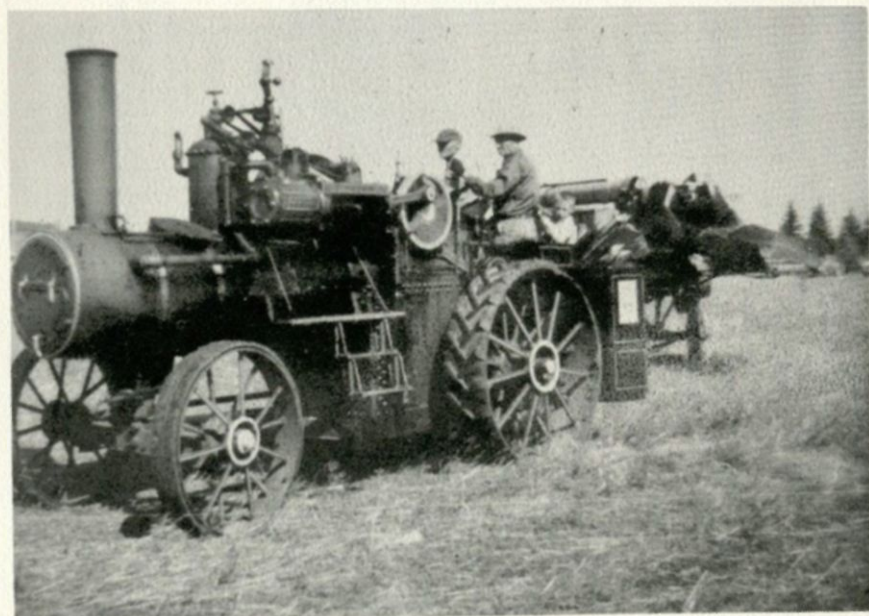
H. P. Lahr's 8 h.p. engine built by Mr. Lahr at St. Joe, Minn.
