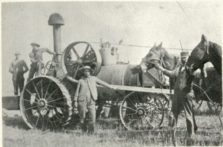
Old threshing scene some 75 years ago. The engine is a Minneapolis steamer. Notice the man holding the horses so they wouldn't run away.
