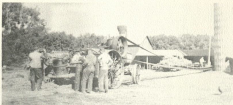
George Melby filling silo with his 22 h.p. Advance engine. Year: 1920. Filling silo at Neely Gray farm at Ashby, Minn.
