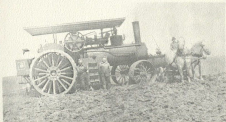
36 h.p. Rumley double cylinder steam engine, plowing prairie sod in Canada. They used 3-ton of coal and 9,000 gallons of water per day, pulling 14 breaker plows. This picture was taken in Canada.
