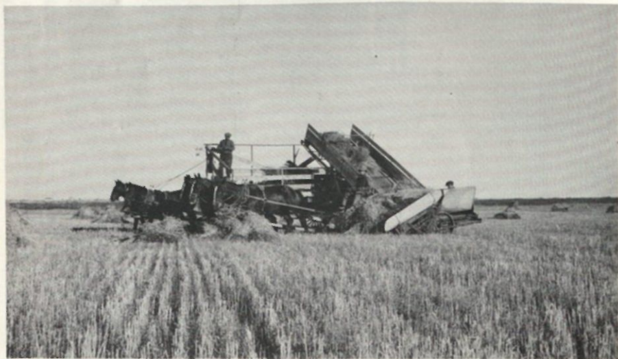
Shock loader loading shocks near Smiley, Sask., Canada. These loaders were used more in Canada than in the U.S. They would load a large load of bundles in a few minutes. They had special racks built for these loaders.
