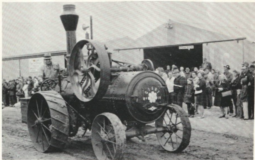
14 H.P. Minnesota Grant steam engine in a parade at the Threshermen's show. Notice the chain drive on the engine. Glenn and Ralph Risbrudt are the proud owners.
