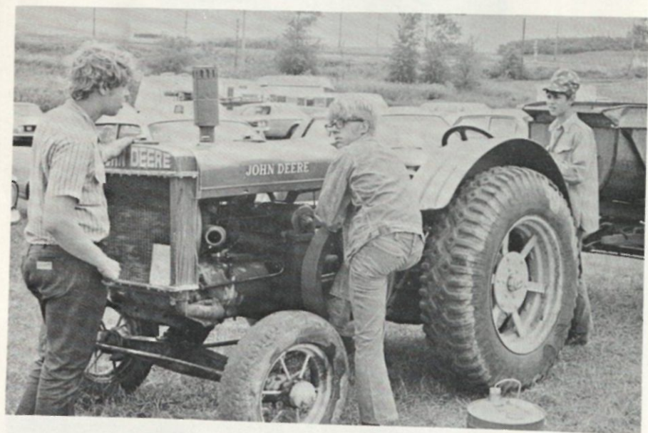
David Schroeder starting his John Deere tractor. It's an old one, see the open spoke flywheel. It was not put on later, either. David restored this tractor and it looks and runs good.
