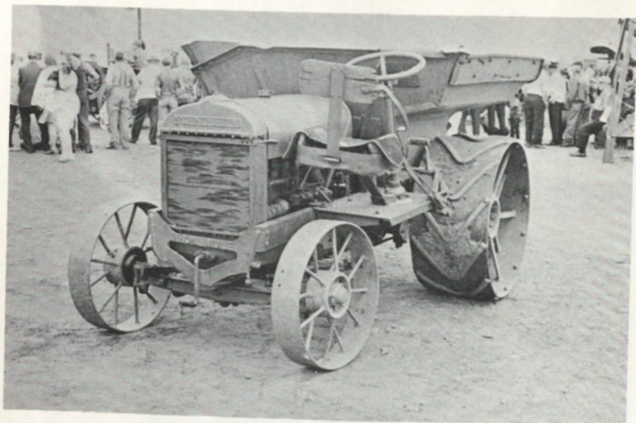
Special dump built on a McCormick Deering tractor. We believe it was used in the coal mines in the Minot, N.D. country. Milton Martinson, owner.
