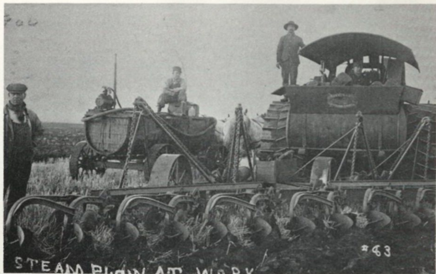
Large Reeves steam engine, plowing at Lakota, N.D. Notice the steam lift plows. Steam was tapped from the engine into cylinders on the plow. This is a 12 bottom plow, picture taken near 1900 the best we can judge. The engine could be a 40 H.P. Cross compound, the largest engine Reeves built.
