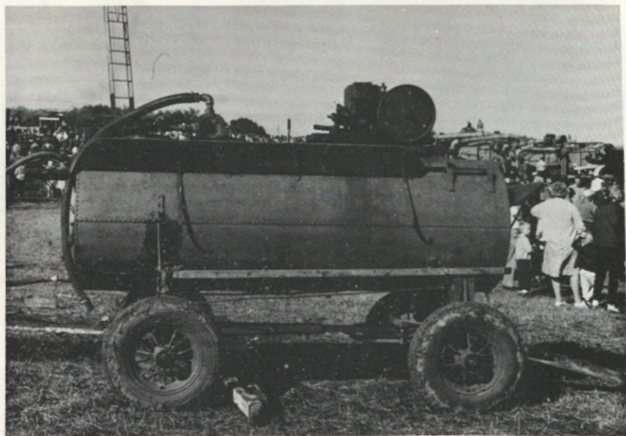
Tank mount on a rubber tired wagon used to haul water for the show. In the olden days the tank man had to pump the water by hand into the tank. This one uses a gasoline engine.
