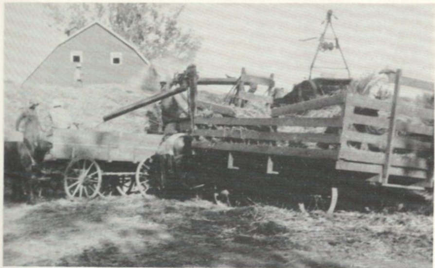
Typical threshing scene. 36-58 Case making a straw stack next to the barn, threshing oats in Iowa.
