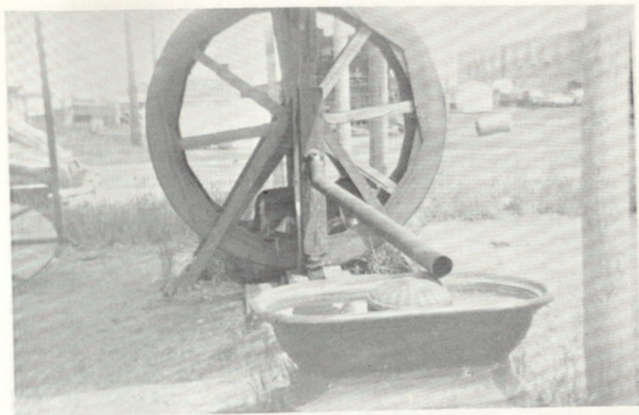
Dog power pumping water at Pioneera. The dogs seemed to like it and would go into the wheel without being told to do it.
