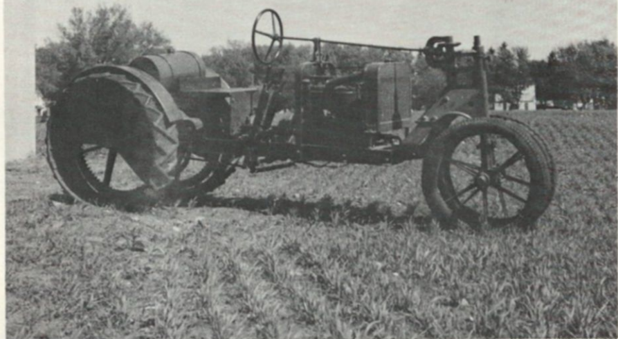
Henry Johnson's 5-10 Avery gas tractor. This is a friction drive tractor and was built in about 1910. As far as we know, it is the only one this size in working order.
