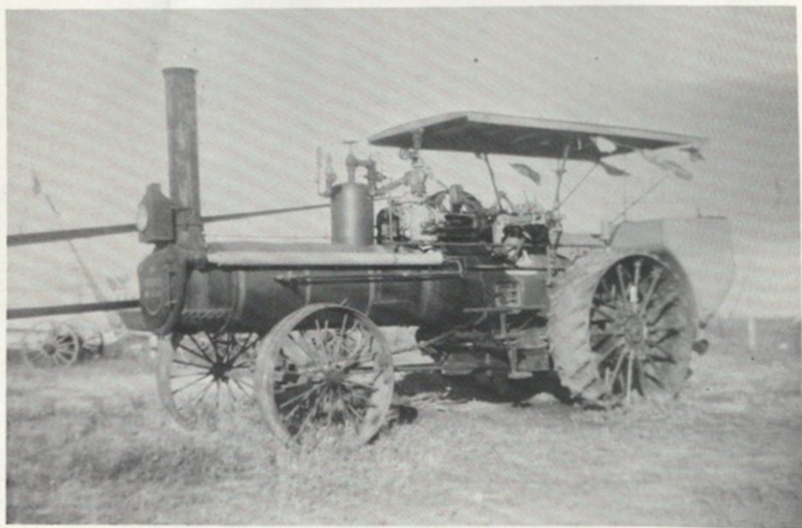
40 H.P. Geeser Peerless steam engine. This is the largest engine this company built. It was used to power the lumber saw mill at Pioneera annual show at Saskatoon, Canada.
