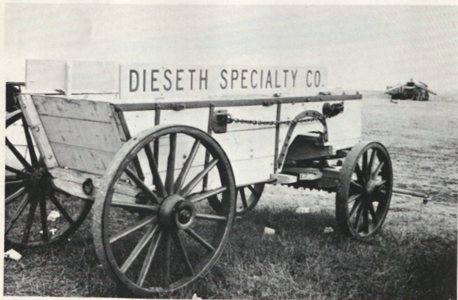
Dump wagon owned by Dieseth Specialty Co., Fergus Falls, Minn. This type of wagon was used in road construction in the pioneer days when horses were used to pull them around.
