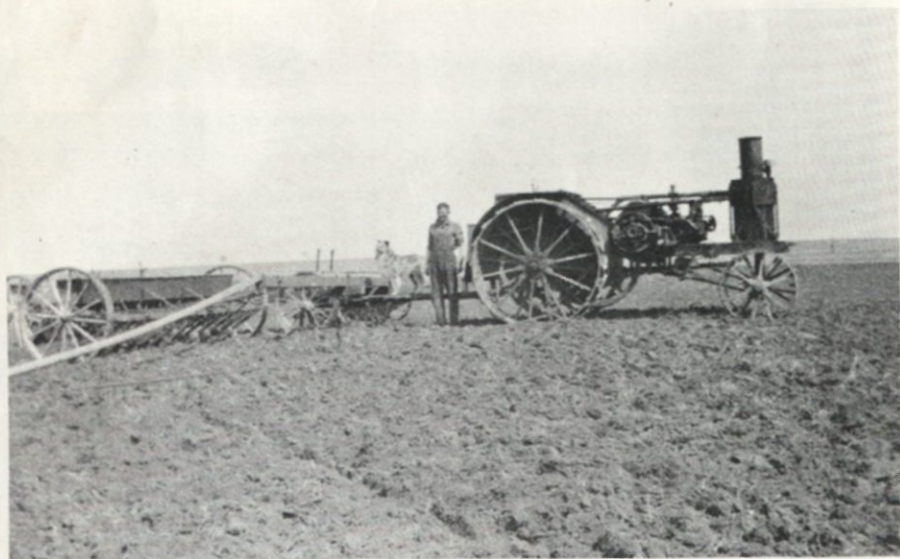
Avery gas tractor pulling three grain drills somewhere in the Dakotas, year could be around 1919.
