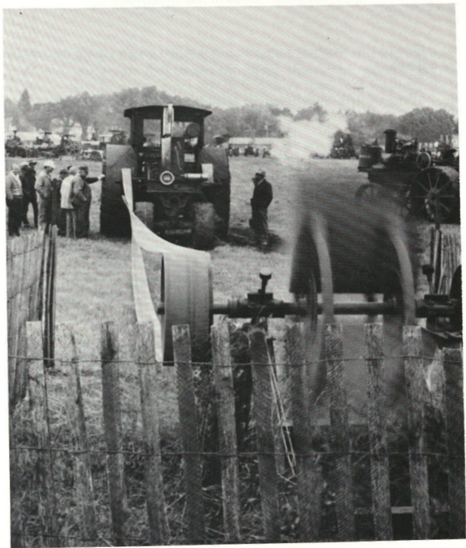
40—80 Minneapolis on the baker fan. These fans give the largest tractor or steam engine a real work out.
