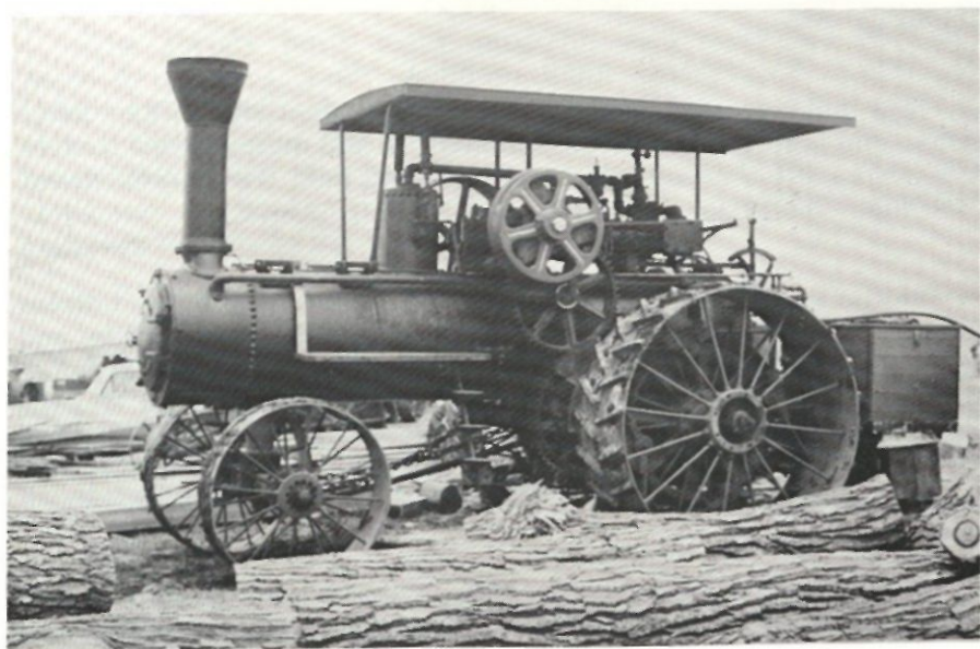
25 h.p. Gaar Scott double cylinder steam engine No. 15206. Built in 1911. Used in the Dalton area since 1919. Used mostly for threshing.
