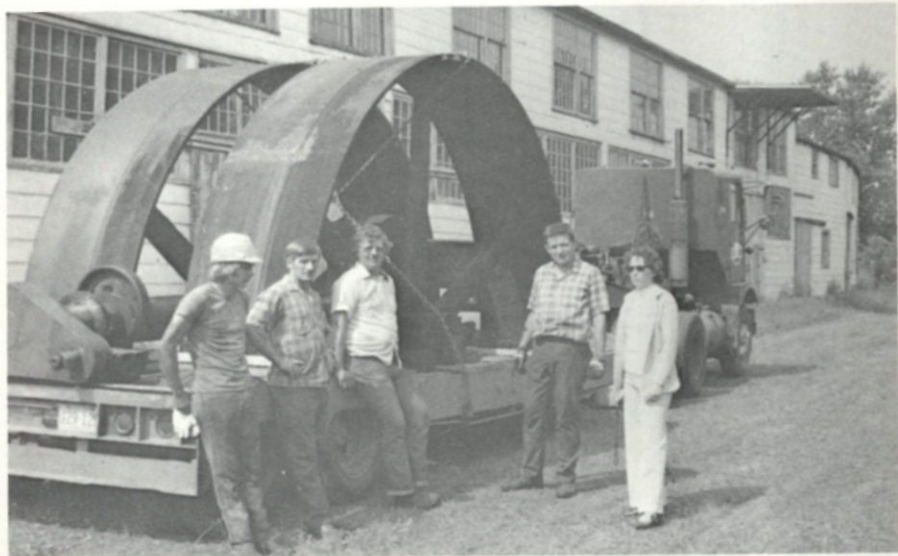
Fly wheel for the big Corliss steam engine loaded at Bay City, Mi. The wheel is 35 inches wide, 15 feet across, weighing 8 ton. The crank shaft is 11 inches in diameter and 12 feet long, weighing 3 ton.
