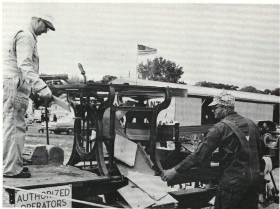
Shingle mill in operation at the show operated by John Nyperud and David Hanson.
