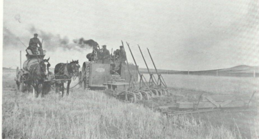
Plowing with a Case engine and an eight bottom plow with drag behind. This picture was taken at Hettinger, N.D., 1913.
