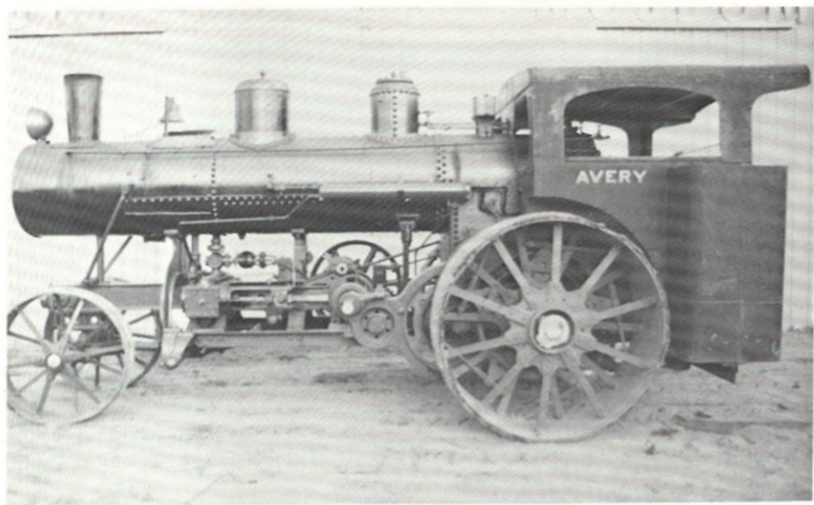
22 h.p. Avery undermounted steam engine about 1910 model owned by Henry Johnson.
