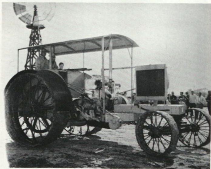
30—60 Russell gas tractor. There are very few of these tractors. We don't believe too many were made. The Russell Company built about 1800 steam engines besides grain separators and tractors.
