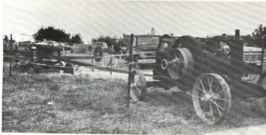
Earl Nelson's 15 h.p. Fairbanks Morse belted to the shingle mill.
