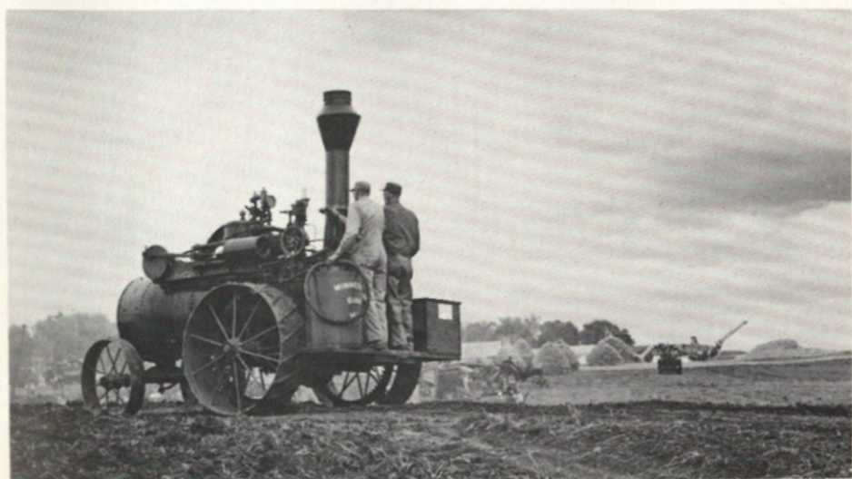
14 h.p. Minnesota Giant owned by Glenn and Ralph Risbrudt. This engine was manufactured by the Minnesota Thresher Manufacturing Co. of Stillwater, Minn. about 1886. The chain drive was the company's first tractor engine, was intended to only haul itself around from place to place. There were several companies making chain drive around this time, but all went to the gear in place of chain.
