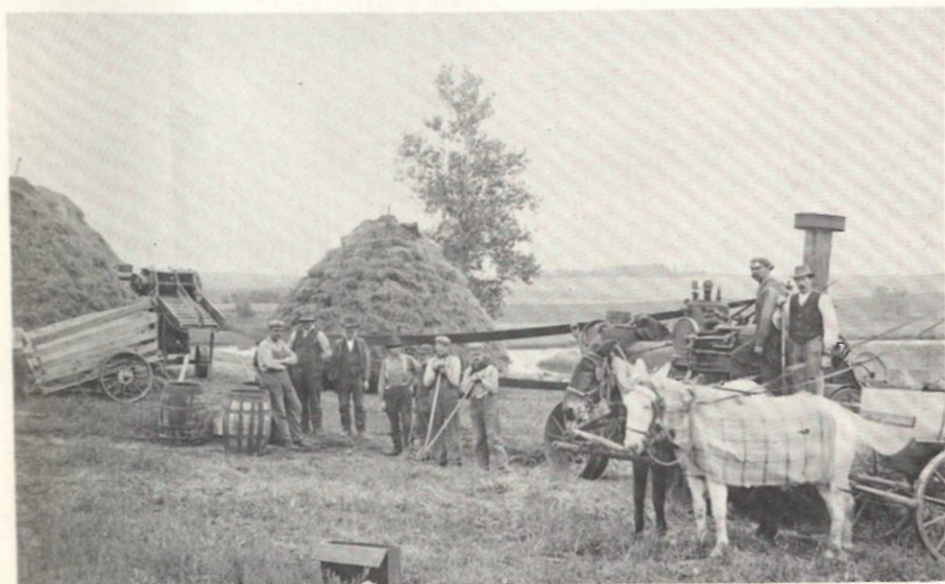
Stack threshing somewhere in Minnesota. See straw cart in front of the grain stack. That was hauled between the engine and separator. Fireman would stand in the cart and used a 3-tined fork to push straw through the firedoor into the firebox. Courtesy Olin Thompson.
