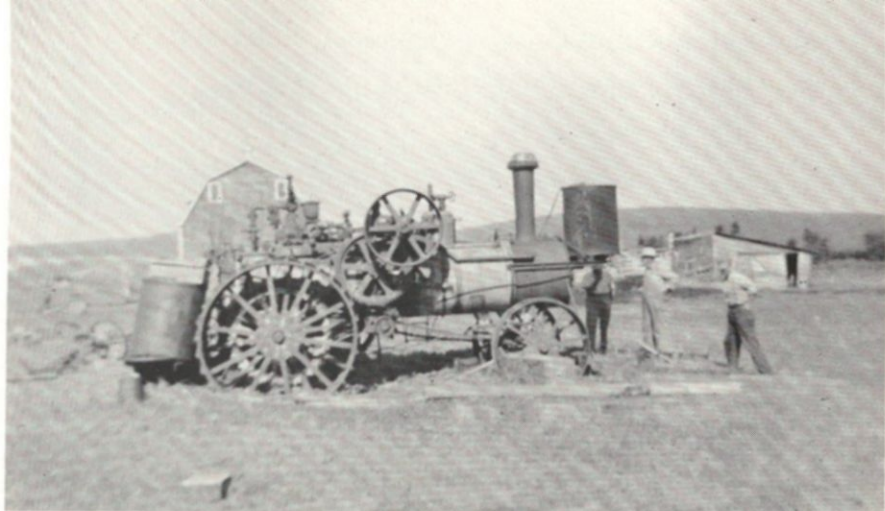
30 h.p. double cylinder, double geared Minneapolis steam engine standing on a farm in western Dakota. It is a very rare machine, as the shafts on the intermediate gear go through a tube in the boiler.
