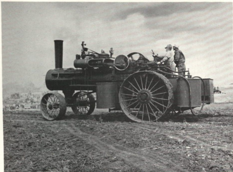
Olin Thompson, engineer and Elton Helleckson on the 25 h.p. Advance Rumley. This is the largest engine the Advance Rumley Co. built.
